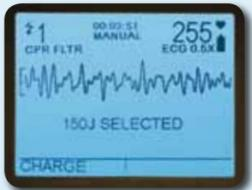
See-Thru CPR filters out compression artifact, which reduces the amount of time without compressions while checking to see whether an organized, shockable rhythm has developed.
