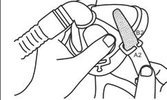
Pull the upper headgear strap A2 through the slot B2 on the mask, making sure the Velcro faces outward.
