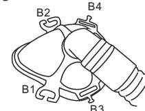
Identify headgear fastening positions on the mask.
