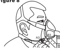
Hook the plastic buckle A3 onto B3 and A4 onto B4 on mask frame.
