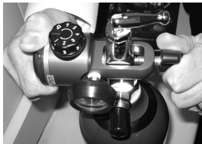
FIGURE 3.1 Attaching the IOCI00P to the Cylinder
