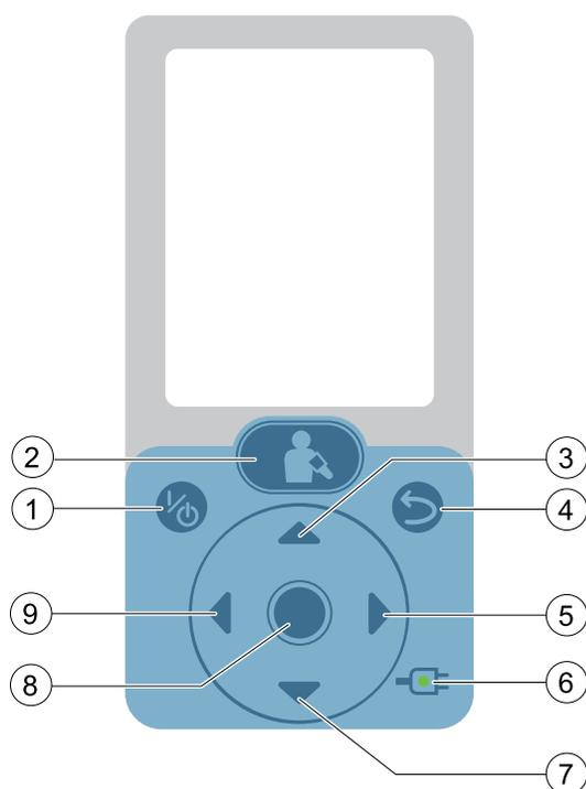
1. **Power on/power off** button: controls power to the device.
